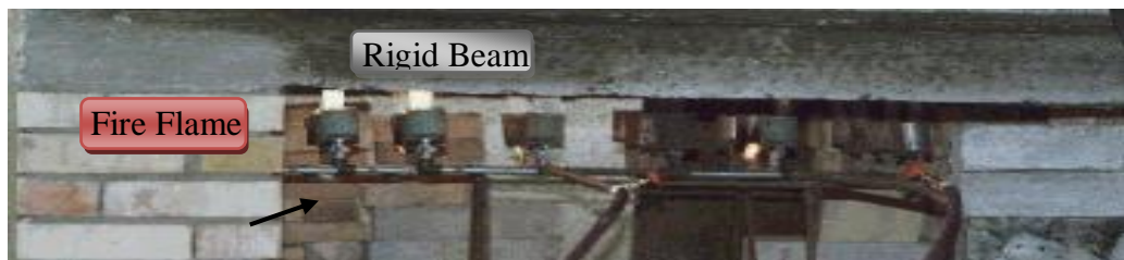
Figure 4. Testing of rigid beam specimens under 25% of ultimate load with exposure to fire flame.
